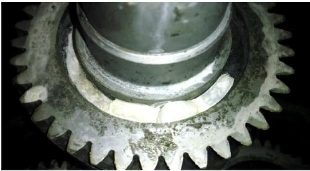
Gears with residue before trial
