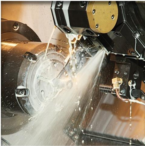
**HOCUT®4800** does not support the growth of bacteria or fungi. The plant manager agreed to try it and added **HOCUT®4800** over top of the old coolant in two systems.
