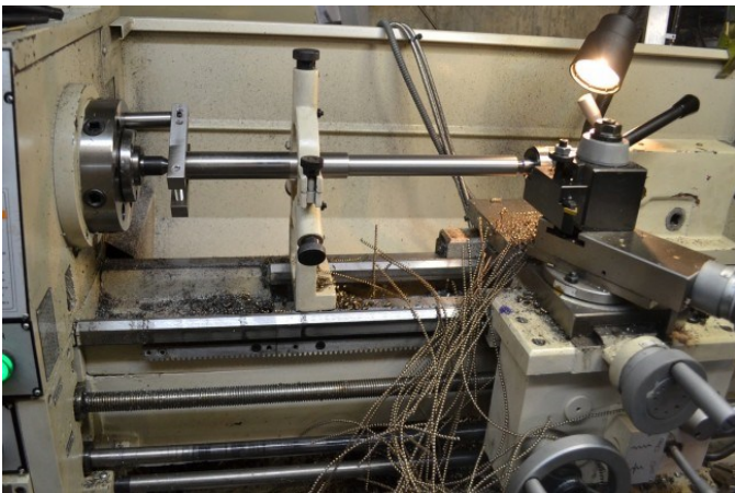
Machining an AR-15 Barrel
